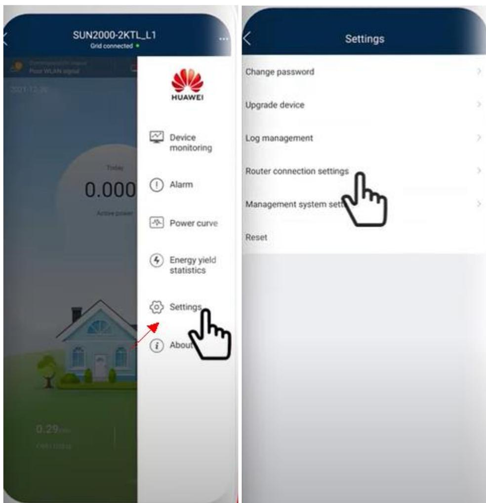
3. After the connection to router is done go one step back and select Management system and press connect:
